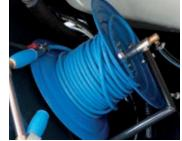
Hose reel with spray gun, working at 15-bar nozzle, for washing the machine. It is connected with the main water pump, using washing circuit water.
